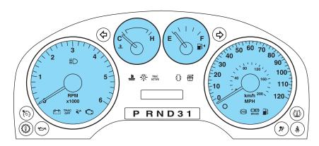
**Speedometer:** Indicates the current vehicle speed.
